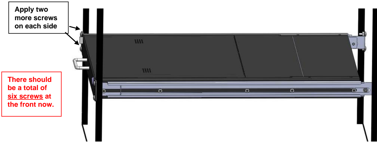
Figure 6- Apply remaining screws to complete installation
