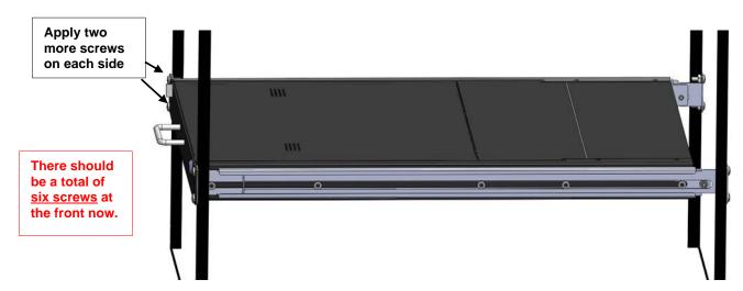
Figure 6- Secure the RACKMUX
