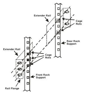
Figure 2- Install cage nuts
