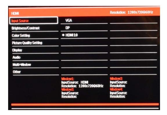
Note: If only one input connector is used, the input source will automatically switch to the active connector. No user selection will be necessary.
