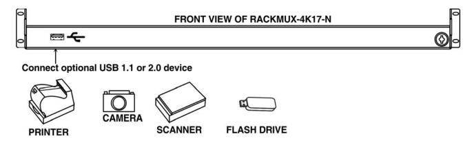
Figure 10- Connect a USB 2.0 device to the front (optional)
