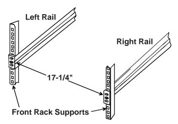
Figure 4- Adjust distance between rails
