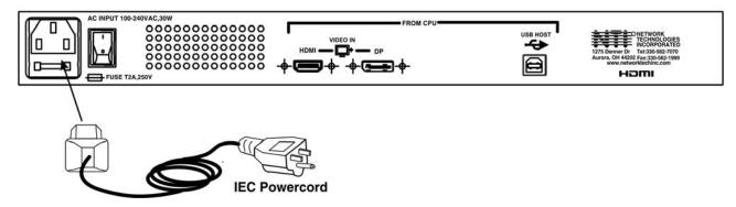
Figure 11- Connect the power cord
