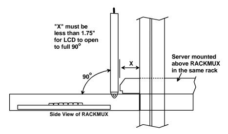
Figure 7- Position RACKMUX with clearance to open
