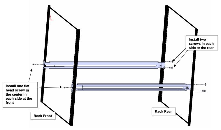
Figure 3- Install rail assemblies
